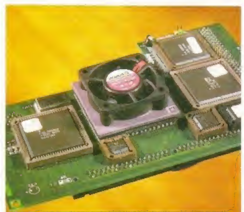
Before you fit a megafast board, like the Falcon, you may need to get rid of your old RAM expansion.
